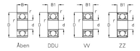
Max rpm ZZ-WW = 32000 В = 6 B1 = 6 r min = 0.3Type = 626 d = 6 D = 19 Load Cor (N) = 885Load Cr (N) = 2340Max rpm DD = 30000
